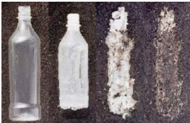
Fig. 5. Various stages of biodegradability of poly films
